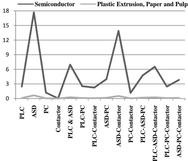
Fig. 7. Benefit-cost ratio when employing equipment level mitigation solutions for semiconductor and plastic extrusion, paper and pulp industries.
