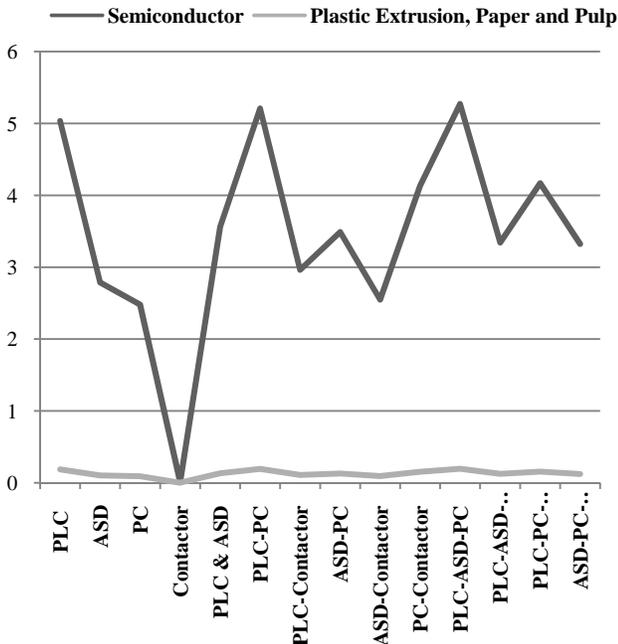
Fig. 8. Benefit-cost ratio when employing control level mitigation solutions for semiconductor and plastic extrusion, paper and pulp industries.
