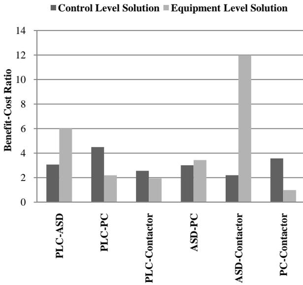
Fig. 3. Benefit-cost ratio when protecting two sensitive equipments.
