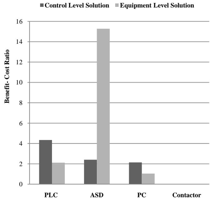
Fig. 2. Benefit-cost ratio when protecting one sensitive equipment.
