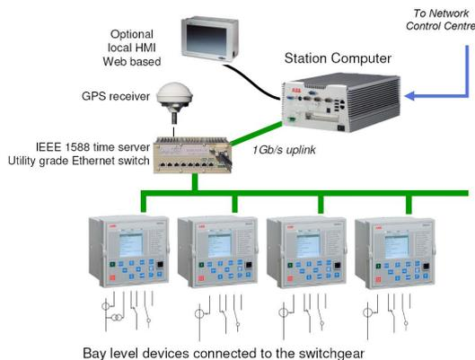
**Figure 1.** Overall setup of centralized protection and control system.
