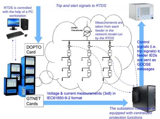
**Figure 3.** RTDS test environment for centralized protection.
