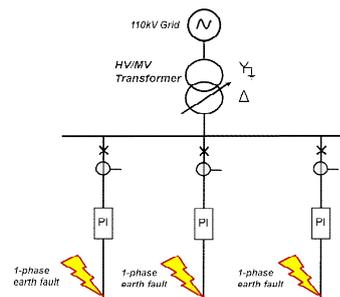
**Figure 2.** MV network modelled using RSCAD.
